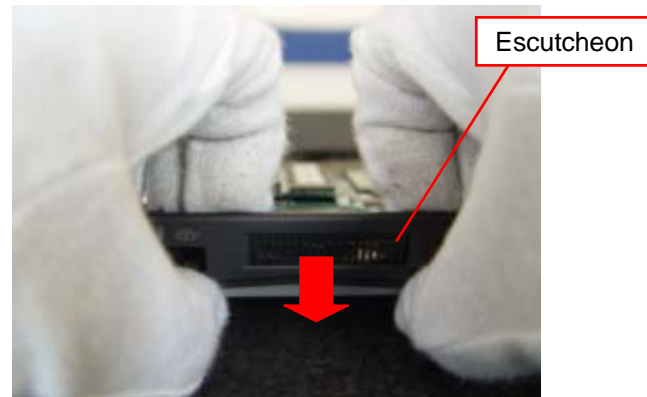
Insert the fingers between the Escutcheon and the Board, outspread the Escutcheon, and disengage the detent.
